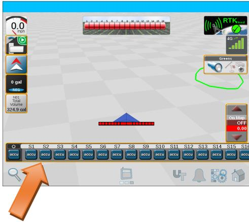
Verify that all of the switches shown on your 'On Screen Switch Box' widget are set to Accu.
