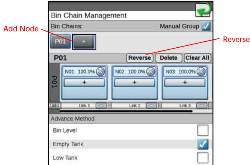
6. Select the advanced method for bin switching. This can either be done when the Bin Level sensor alarm is triggered, when there is an empty tank, or a low tank alarm is triggered.
