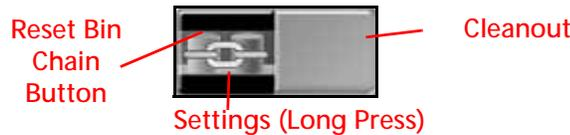
To reset the chain to the first link, press the left half of the Bin Chain button.
