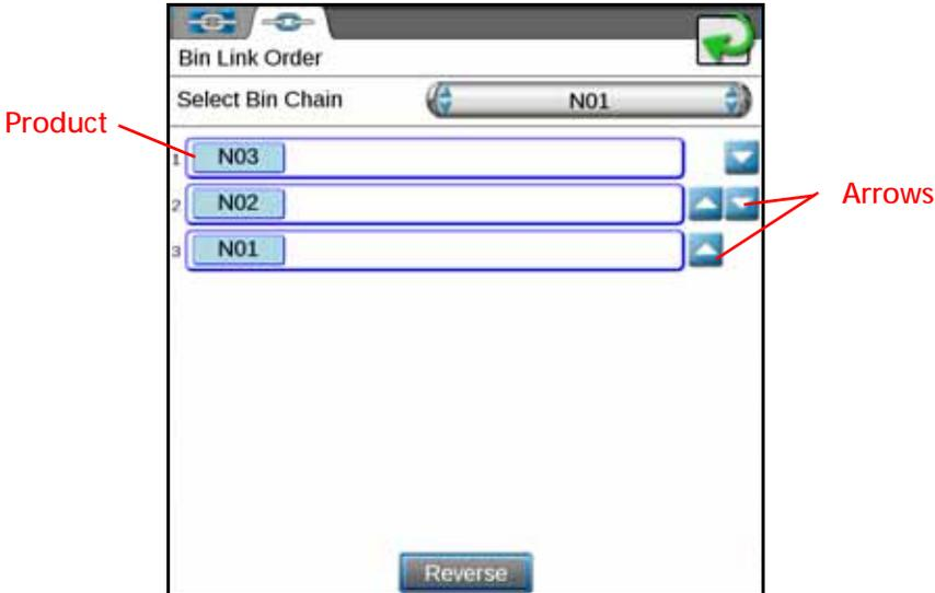
2. Once complete, press the back arrow to save the settings. If desired, press Reverse to reset the order to the previously ran job.
