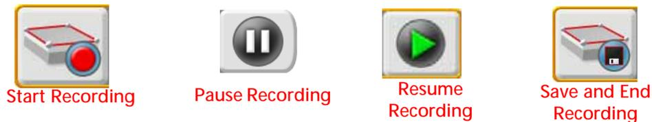
1. Touch the Start Recording button shown on the scouting widget to begin recording the field feature. ROS will automatically capture points along the path driven by the equipment.
