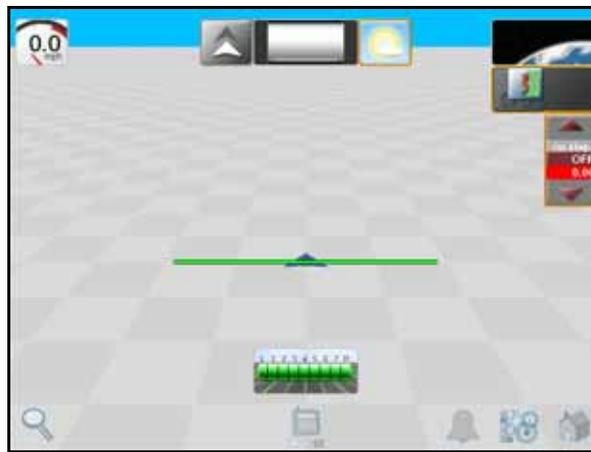
ROS allows each equipment operator to select which widgets will be displayed during operation, move each of the widgets to a desired portion of the screen, and save multiple screen configurations for use during future operations and other operators.
