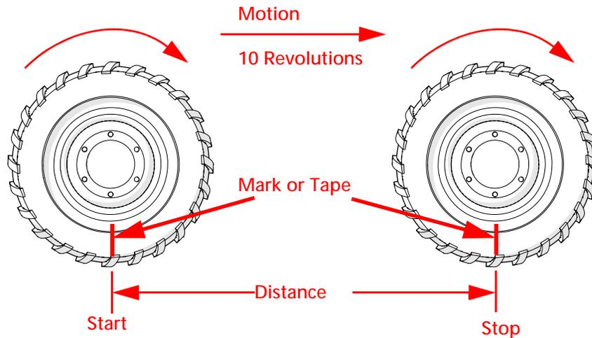
4. Mark the stopping point and measure the distance between the starting and stopping marks on the ground in inches [dm]. Round to the nearest whole number.
