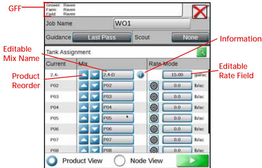
**NOTE:** Select the Node View radio button to view the node name and the current mix.
